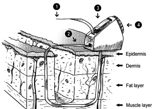
FIG. 2. Schematic drawing of the Wisebands wound closure device: 1, A 5-mm-wide polypropylene band; 2, the "in port" at the base of the device; 3, safety catch; 4, rotating knob. Rotating the knob (4) on the device applies controlled load to the band (1), causing gradual traction and tension on the tissue. The band exits from the device through an exit port on the top of the device.
